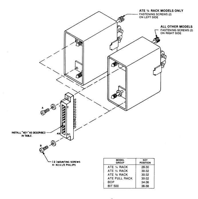
FIG. 1 INSTALLATION OF THE PC-12 MATING CONNECTOR
